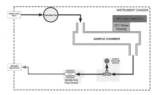
Figure 3-20: GFC7001T/GFC7001TM Internal Gas Flow
